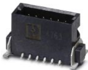
SMD male connector, Nominal current at 20 °C: 1.4 A, Test voltage: 500 V AC, number of positions: 20, pitch: 1.27 mm, color: black, contact surface: Gold, mounting: SMD soldering
