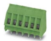
PCB terminal block, nominal current: 24 A, rated voltage (III/2): 400 V, nominal cross section: 2.5 mm², pitch: 5.08 mm, number of positions: 5, connection method: Screw connection with tension sleeve, mounting: Wave soldering, conductor/PCB connection direction: 55 °, color: green, Pin layout: Linear pinning, Solder pin [P]: 4.5 mm. The article can be aligned to create different nos. of positions!
