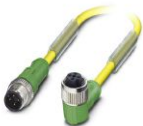
Sensor/actuator cable, 4-position, PUR/PVC, yellow, Plug straight M12, coding: A, on Socket angled M12, coding: A, cable length: 1.5 m, DESINA
