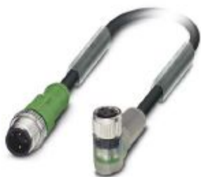
Sensor/actuator cable, 3-position, PUR halogen-free, black-gray RAL 7021, Plug straight M12, coding: A, on Socket angled M8, with 2 LEDs, cable length: 0.3 m
