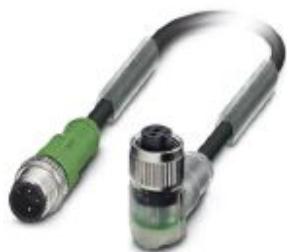
Sensor/actuator cable, 3-position, PUR halogen-free, black-gray RAL 7021, Plug straight M12, coding: A, on Socket angled M12, coding: A, with 2 LEDs, cable length: 3 m
