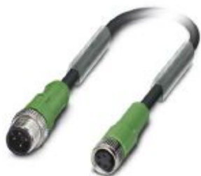
Sensor/actuator cable, 4-position, PUR halogen-free, black-gray RAL 7021, Plug straight M12, coding: A, on Socket straight M8, cable length: 0.6 m
