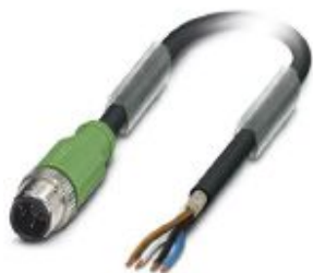
Sensor/actuator cable, 4-position, PUR halogen-free, black-gray RAL 7021, shielded, Plug straight M12, coding: A, on free cable end, cable length: 1.5 m
