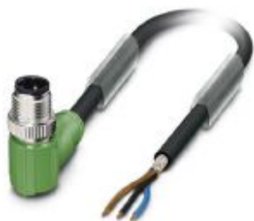
Sensor/actuator cable, 3-position, PUR halogen-free, black-gray RAL 7021, shielded, Plug angled M12, coding: A, on free cable end, cable length: 5 m
