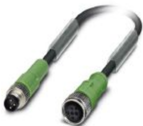
Sensor/actuator cable, 3-position, PUR halogen-free, black-gray RAL 7021, Plug straight M8, on Socket straight M12, coding: A, cable length: 0.3 m
