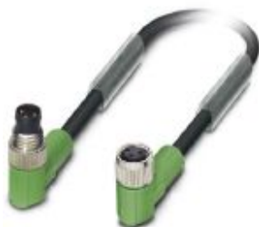
Sensor/actuator cable, 3-position, PUR halogen-free, black-gray RAL 7021, Plug angled M8, on Socket angled M8, cable length: 1.5 m
