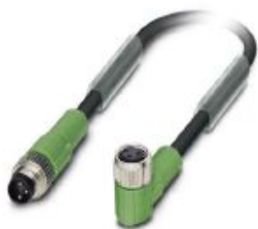
Sensor/actuator cable, 3-position, PUR halogen-free, black-gray RAL 7021, Plug straight M8, on Socket angled M8, cable length: 0.3 m
