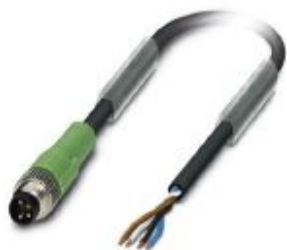
Sensor/actuator cable, 4-position, PUR halogen-free, black-gray RAL 7021, Plug straight M8, on free cable end, cable length: 5 m
