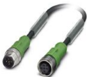
Sensor/actuator cable, 5-position, PUR halogen-free, black-gray RAL 7021, Plug straight M12, coding: A, on Socket straight M12, coding: A, cable length: 0.6 m
