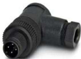
Connector, Universal, 4-position, Plug angled M12, Coding: A, Screw connection, knurl material: Plastic, cable gland Pg7, external cable diameter 4 mm ... 6 mm
