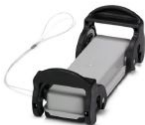
Protective cover B24, with double locking latch, protective cover material: PA, height: 21.6 mm, seal: yes, with lanyard, diameter of retaining cord eyelet: 30 mm
