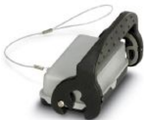
Protective cover B10, with single locking latch, protective cover material: PA, height: 21.6 mm, seal: yes, with lanyard, diameter of retaining cord eyelet: 30 mm
