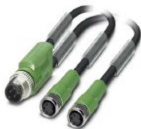
Sensor/actuator cable, 3-position, PUR halogen-free, black-gray RAL 7021, Plug straight M12, coding: A, on Socket straight M8 and Socket straight M8, coding: A, cable length: 0.3 m
