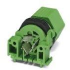
Panel feed-through, for internal wall mounting, with dip-solder connection, length of the solder pin: 3.8 mm, hole  $\varnothing$  2-pos. = 19.0 mm - 0.3 mm
