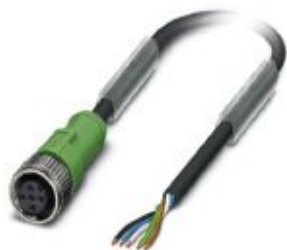
Sensor/actuator cable, 5-position, PUR halogen-free, black-gray RAL 7021, free cable end, on Socket straight M12, coding: A, cable length: 1.5 m
