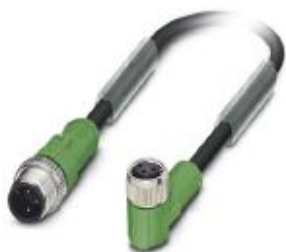
Sensor/actuator cable, 3-position, PUR halogen-free, black-gray RAL 7021, Plug straight M12, coding: A, on Socket angled M8, cable length: 0.6 m
