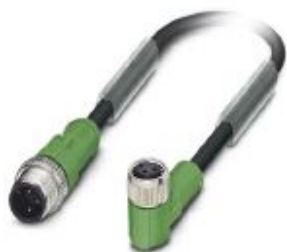
Sensor/actuator cable, 3-position, PUR halogen-free, black-gray RAL 7021, Plug straight M12, coding: A, on Socket angled M8, cable length: 0.3 m
