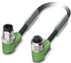
Sensor/actuator cable, 4-position, PUR halogen-free, black-gray RAL 7021, Plug angled M12, coding: A, on Socket angled M12, coding: A, cable length: 1.5 m
