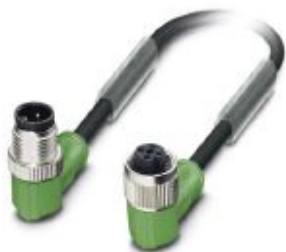
Sensor/actuator cable, 3-position, PUR halogen-free, black-gray RAL 7021, Plug angled M12, coding: A, on Socket angled M12, coding: A, PIN 2+4 bridged, cable length: 3 m
