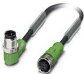
Sensor/actuator cable, 3-position, PUR halogen-free, black-gray RAL 7021, Plug angled M12, coding: A, on Socket straight M12, coding: A, PIN 2+4 bridged, cable length: 0.3 m
