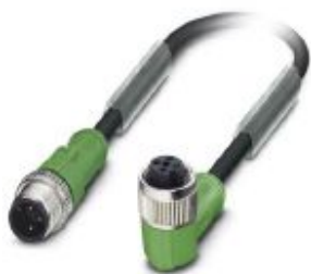
Sensor/actuator cable, 3-position, PUR halogen-free, black-gray RAL 7021, Plug straight M12, coding: A, on Socket angled M12, coding: A, PIN 2+4 bridged, cable length: 0.6 m
