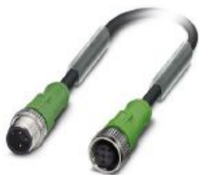
Sensor/actuator cable, 3-position, PUR halogen-free, black-gray RAL 7021, Plug straight M12, coding: A, on Socket straight M12, coding: A, PIN 2+4 bridged, cable length: 1.5 m
