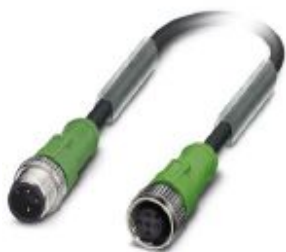
Sensor/actuator cable, 3-position, PUR halogen-free, black-gray RAL 7021, Plug straight M12, coding: A, on Socket straight M12, coding: A, PIN 2+4 bridged, cable length: 0.6 m
