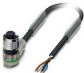
Sensor/actuator cable, 4-position, PUR halogen-free, black-gray RAL 7021, free cable end, on Socket angled M12, coding: A, with 3 LEDs, cable length: 5 m
