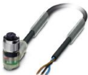
Sensor/actuator cable, 3-position, PUR halogen-free, black-gray RAL 7021, free cable end, with 2 LEDs, PIN 2+4 bridged, on Socket angled M12, coding: A, with 2 LEDs, PIN 2+4 bridged, cable length: 3 m
