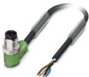
Sensor/actuator cable, 4-position, PUR halogen-free, black-gray RAL 7021, Plug angled M12, coding: A, on free cable end, cable length: 5 m
