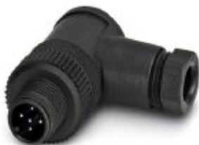
Connector, Universal, 5-position, Plug angled M12, Coding: A, Screw connection, knurl material: Plastic, cable gland Pg7, external cable diameter 4 mm ... 6 mm
