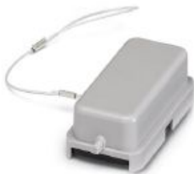
Protective cover D15, for single locking latch, protective cover material: PA, height: 20.5 mm, seal: yes, with lanyard, diameter of retaining cord eyelet: 30 mm
