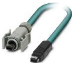
Assembled FireWire cable, shielded, color: RAL 5021 (water blue), PUR outer sheath, FireWire/IP67 on FireWire/standard, length: 2 m
