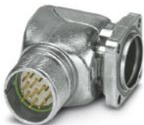
Device connector for front wall, RC, angled rotatable, shielded: yes, for standard and SPEEDCON interlock, M23, No. of pos.: 12, type of contact: Pin, Crimp connection, Axial O-ring, 4x Ø 3.2
