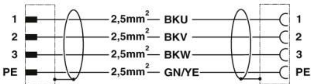
Contact assignment of M17 plugs/sockets
