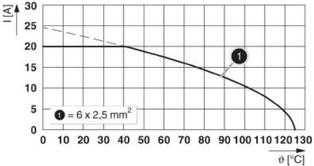
I = current strength,  $\vartheta$  = ambient temperature, 6x 20 A
