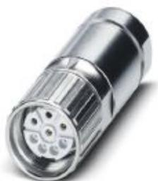
Cable connector, straight long, Screw locking, M23, number of positions: 5+PE, type of contact: Socket, shielded: yes, cable diameter range: 7.5 mm ... 18 mm, number of positions: 6, connection method: Crimp connection
