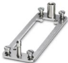
Docking frame for racks, for contact inserts of B24 type, with four M5 flat headed screws, rack balance x/y axis \pm 1.5 mm
