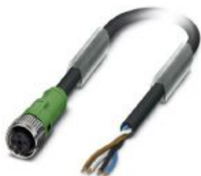
Sensor/actuator cable, 4-position, PUR, black-gray RAL 7021, free cable end, on Socket straight M12 SPEEDCON, coding: A, cable length: 15 m
