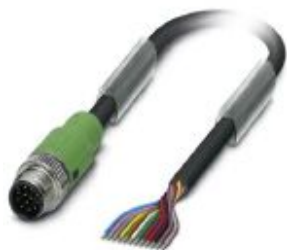
Sensor/actuator cable, 12-position, PVC, black RAL 9005, Plug straight M12 SPEEDCON, coding: A, on free cable end, cable length: 3 m
