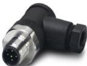
Connector, 5-position, Plug angled M12, Coding: A, Screw connection, knurl material: Stainless steel 1.4404, cable gland Pg7, external cable diameter 4 mm ... 6 mm
