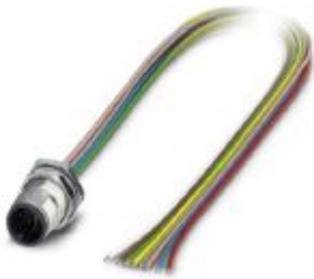
Sensor/actuator flush-type plug, 8-pos., M12 SPEEDCON, rear/screw mounting with M12 thread, with 0.5 m TPE litz wire, 8 x 0.25 mm 2
