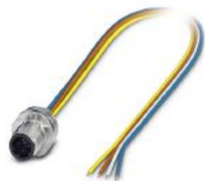
Bus system flat-type plug, PROFINET, 4-position, Plug, straight, M12-SPEEDCON, D-coded, Front mounting, M16 x 1.5, Individual wires, cable length: 0.5 m, 0.34 mm², TPE litz wire
