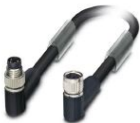
Bus system cable, INTERBUS, 4-position, PUR halogen-free, black RAL 9005, shielded, Plug angled M8, on Socket angled M8, cable length: 1 m
