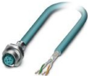
Bus system flush-type socket, Ethernet, 4-pos., M12, shielded, D-coded, rear/screw mounting with M16 thread, with 5 m bus cable, 2 x 2 x 0.14 mm 2
