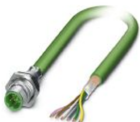
Bus system flush-type male connector, INTERBUS, 5-pos., M12, shielded, B-coded, rear/screw mounting with M16 thread, with 1 m bus line
