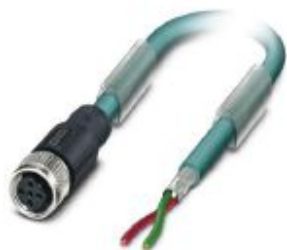
Bus system cable, PROFIBUS, 2-position, PUR/PVC, blue, shielded, free cable end, on Socket straight M12, coding: B, cable length: 5 m
