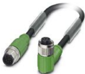
Sensor/actuator cable, 8-position, PUR halogen-free, black-gray RAL 7021, shielded, Plug straight M12, coding: A, on Socket angled M12, coding: A, cable length: 0.6 m
