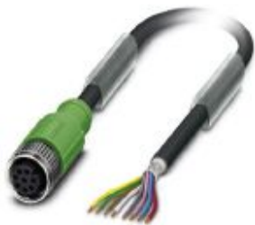
Sensor/actuator cable, 8-position, PUR halogen-free, black-gray RAL 7021, shielded, free cable end, on Socket straight M12, coding: A, cable length: 3 m
