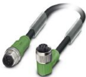
Sensor/actuator cable, 8-position, PUR halogen-free, black-gray RAL 7021, Plug straight M12, coding: A, on Socket angled M12, coding: A, cable length: 3 m
