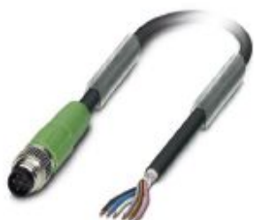
Sensor/actuator cable, 6-position, PUR halogen-free, black-gray RAL 7021, shielded, Plug straight M8, on free cable end, cable length: 10 m
